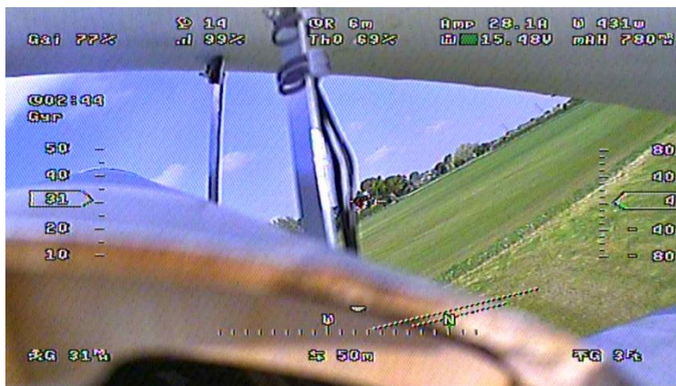
View forwards down the nose of an SE5a rolling to right after takeoff. OSD gives speed in mph on left ladder and height on right in feet.
